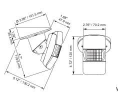
Ceiling mounts to a round 3.0 mud-ring using the celing mount adapter
