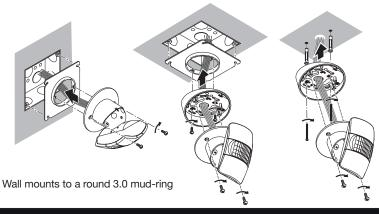
Can be mounted directly to the ceiling or wall using anchor bolts or can be mounted to the ceiling using the supplied 1/2" snap in chase nipple, washer and lock nut. When mounting to the ceiling, the ceiling mount adapter should be used.
