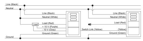
(Master / Master) Three-way Wiring - up to maximum 4 sensors can be grouped via Switch Link
