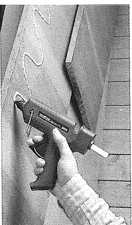
Large surface require a generous spread of glue (e. g.: wavy lines).
