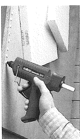
Also hard foam can be glued without problem as long as the glue is placed on the carrier material and not on the polystyrene (e. g. drops).
